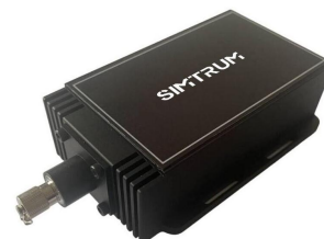
Si-APD Ultra-sensitive photodetector (VIS-NIR)
